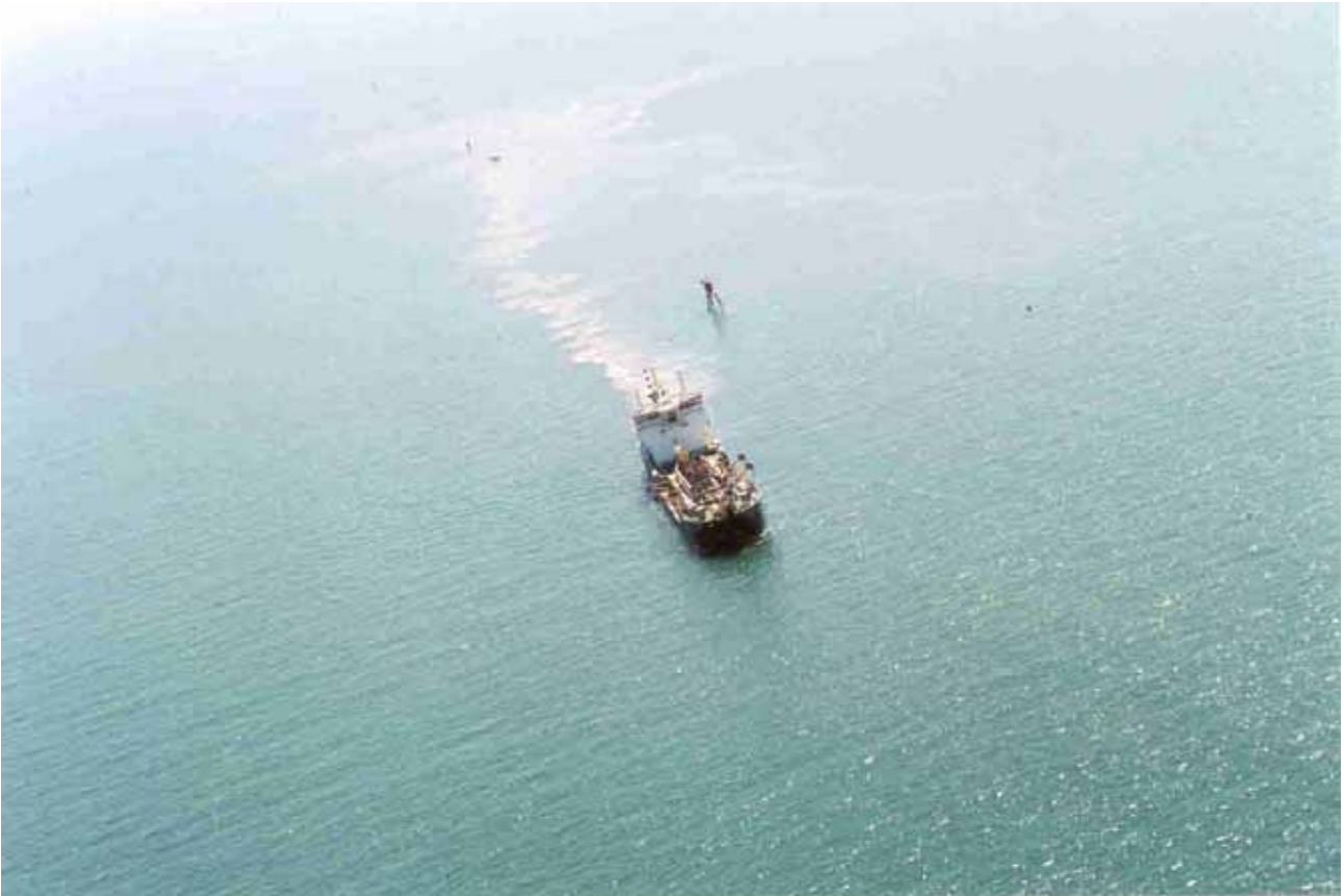
Plate 7: Overall view of turbidity plume from Brisbane during dredging on return leg into Port. Beacon 12 foreground, with survey vessel and beacon 10 in background.
