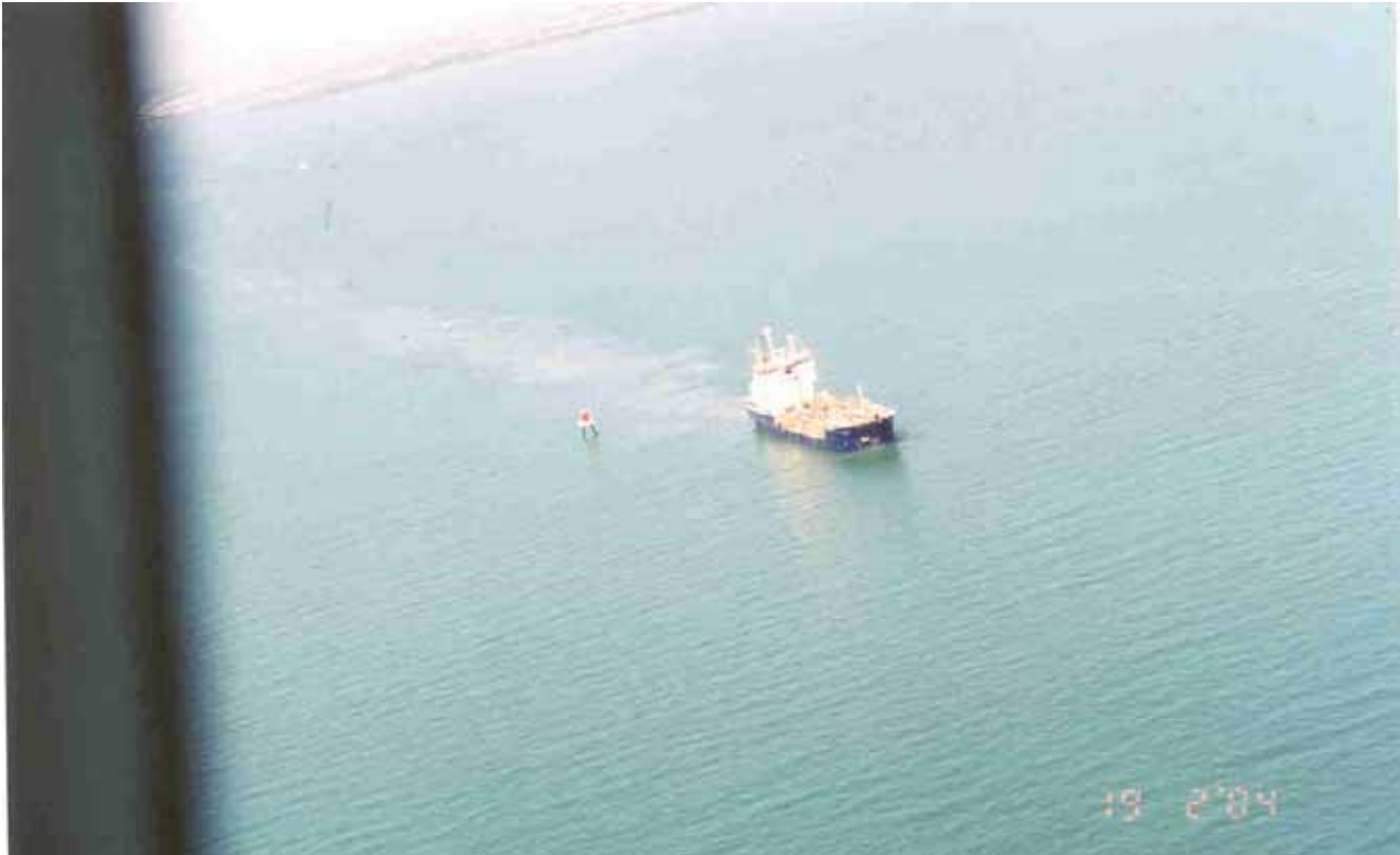
Plate 1: Brisbane dredging the east toeline of the Outer Bar Cutting in a seaward direction. Overall view shows dredging plume before and just after start of hopper overflow. Plates 1 to 10 refer to dredging activities on the 19 February 2004.
