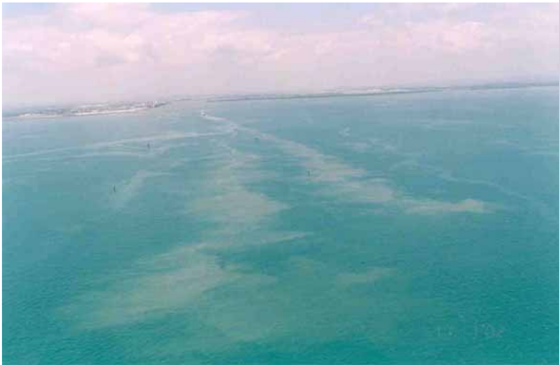
Plates 11 and 12 showing the size and shape of dredging plumes associated with operation of the Brisbane on the ebb tide of 11 th January 2002.
