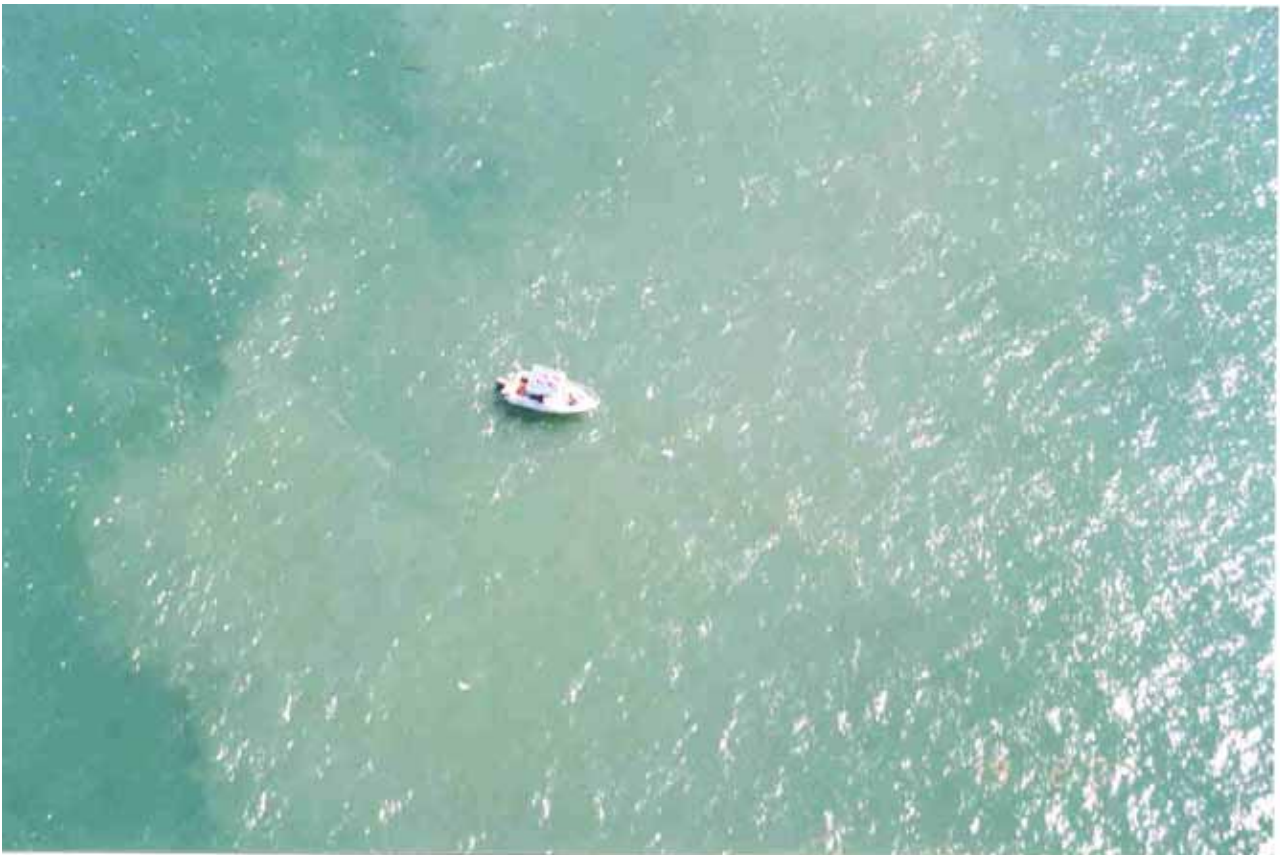
Plate 3: Close up view of dredge plume before hopper overflow.
