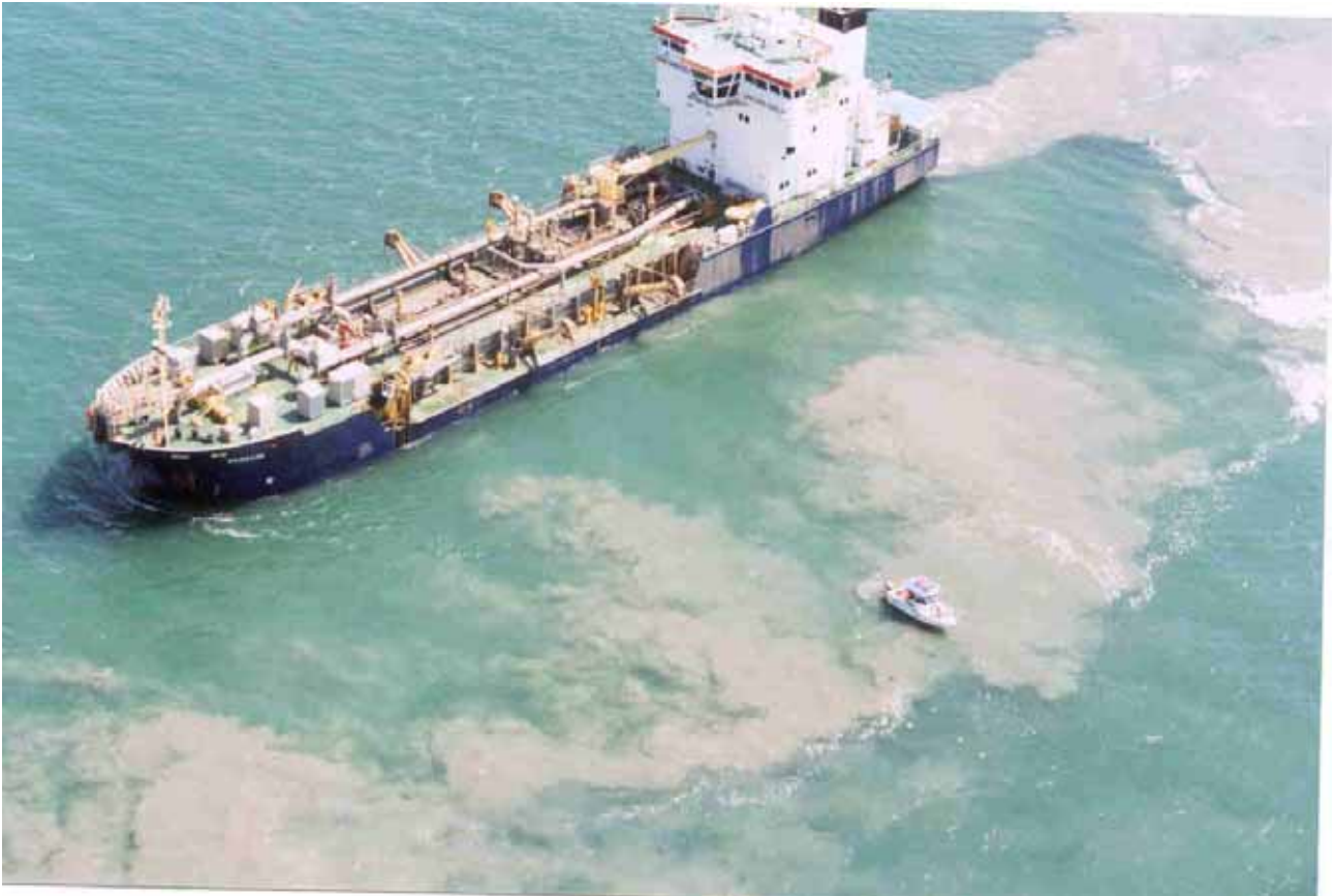
Plate 5: Dredge plume from hopper overflow just after Brisbane turns and begins to dredge back into Port. Survey vessel in foreground, with crew collecting water samples.
