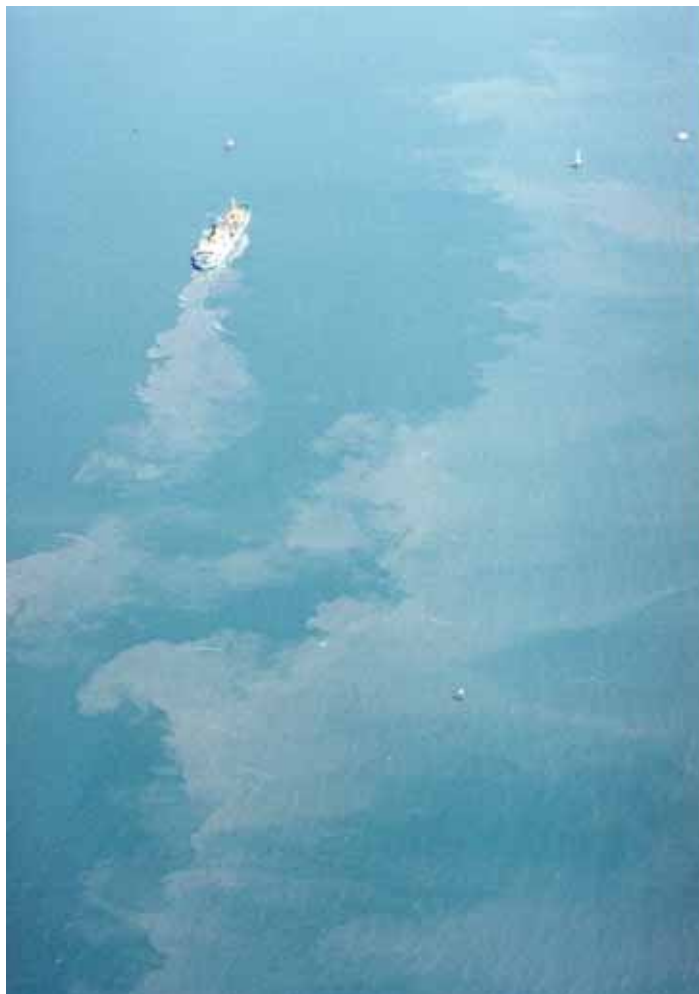
Plates 13 and 14 showing the comparative size and shape of dredging plumes associated with operation of the Sir Thomas Hiley on the ebb tide of 27 th September 1995.
