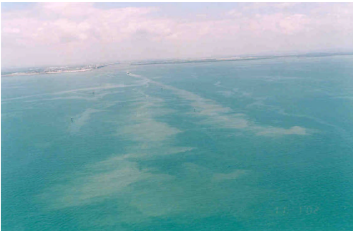
Plate 2 showing the northward movement of the turbid plumes resulting from the hopper overflow from the dredger Brisbane on the ebb tide.
