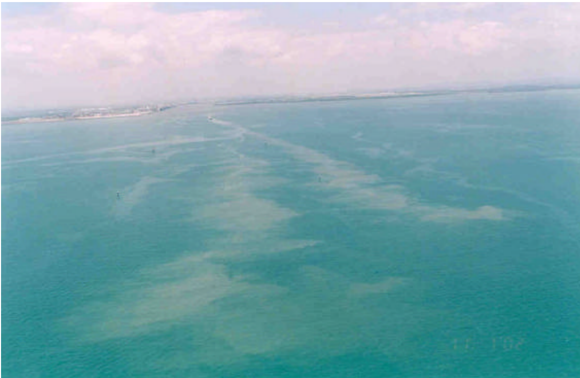
Plates 5 and 6 showing the size and shape of dredging plumes associated with operation of the Brisbane on the ebb tide of 11 th January 2002.
