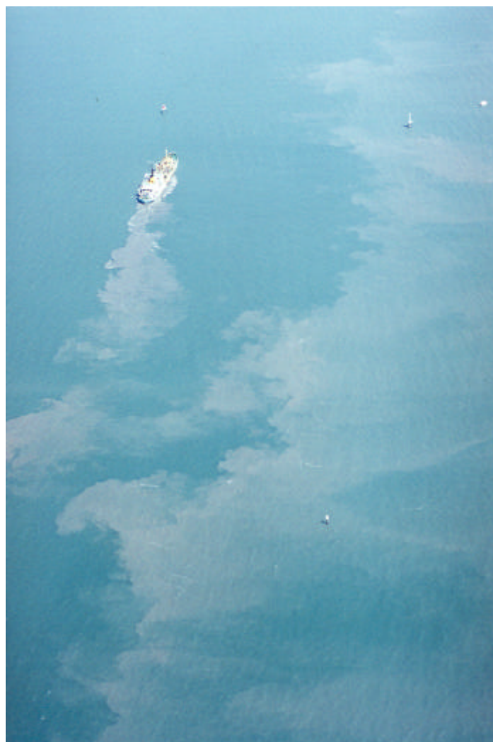
Plates 7 and 8 showing the comparative size and shape of dredging plumes associated with operation of the Sir Thomas Hiley on the ebb tide of 27 th September 1995.
