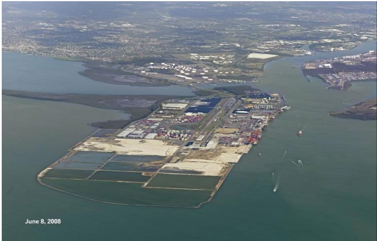
Figure 4 Future Port Expansion oblique aerial dated June 2008. Note the completion of inner bund walls for ponds R3, C3 and B3.
