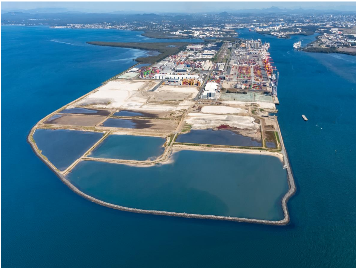
Figure 6 Future Port Expansions oblique aerial updated July 2014. Note the completion of inner bund wall for paddock B4
