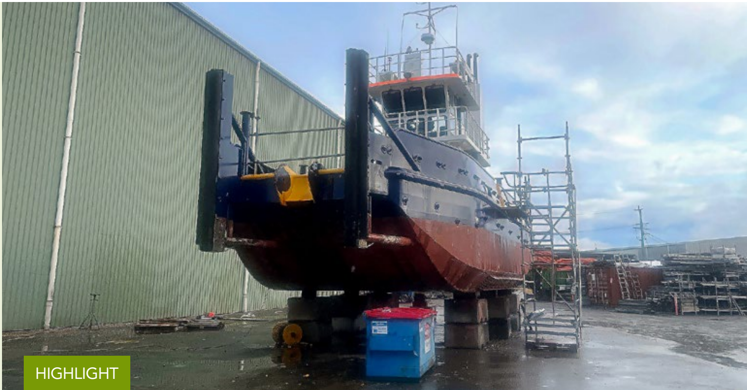
Repurposing used rubber fender material for the Frank Wilson vessel
