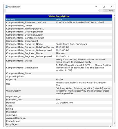
Figure 6 Extract from the GIS of the information the Port has on the existing line. Note this has been surveyed, so its location is accurate.
