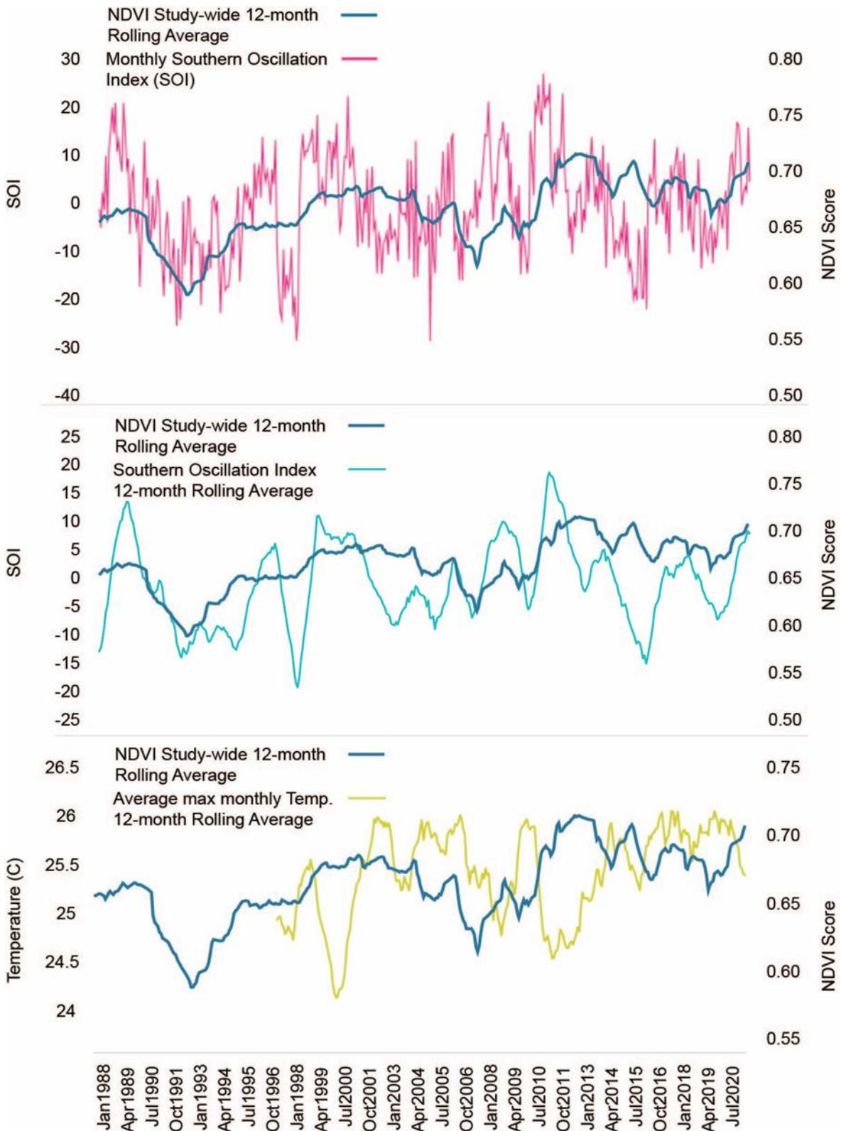
Figure 3.13 Relationships between the 12 month rolling average of NDVI score and: monthly Southern Oscillation Index (SOI) (top); 12 month rolling average of SOI (middle); and the rolling average of maximum monthly temperature (bottom)
