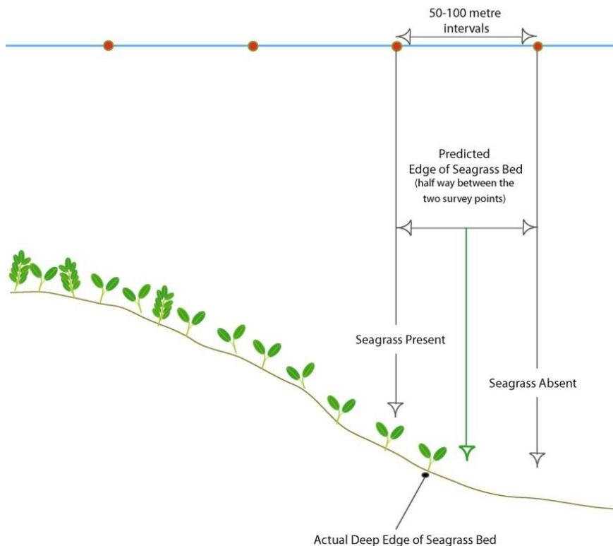
Figure 3-2 Permanent survey point method for identifying the edge of seagrass meadow
