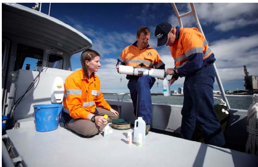
Figure 3-2: Niskin water sampler used for water sample collection.
