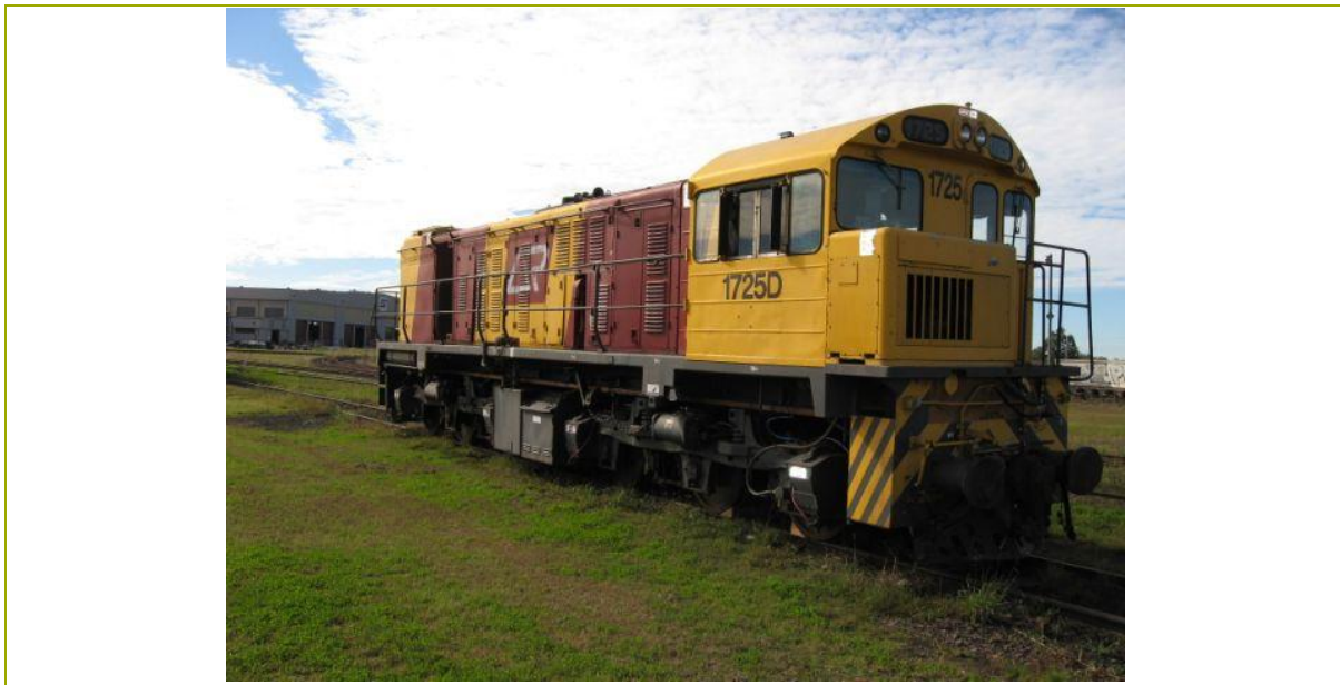
Figure 5.1: A 1150 Hp, 8 Cylinder 2-Stroke Diesel Shunting Locomotive
