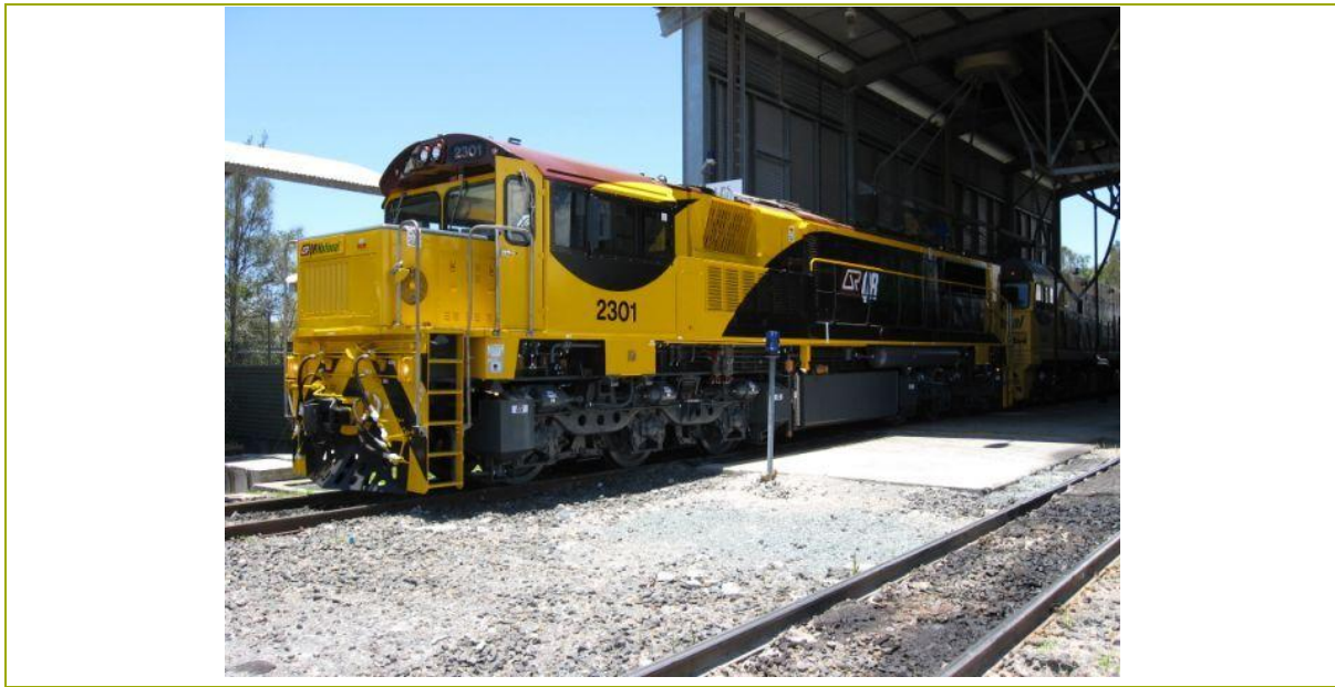
Figure 5.2: A 2,300 Hp 12 Cylinder 2-Stroke Diesel Turbo Locomotive
