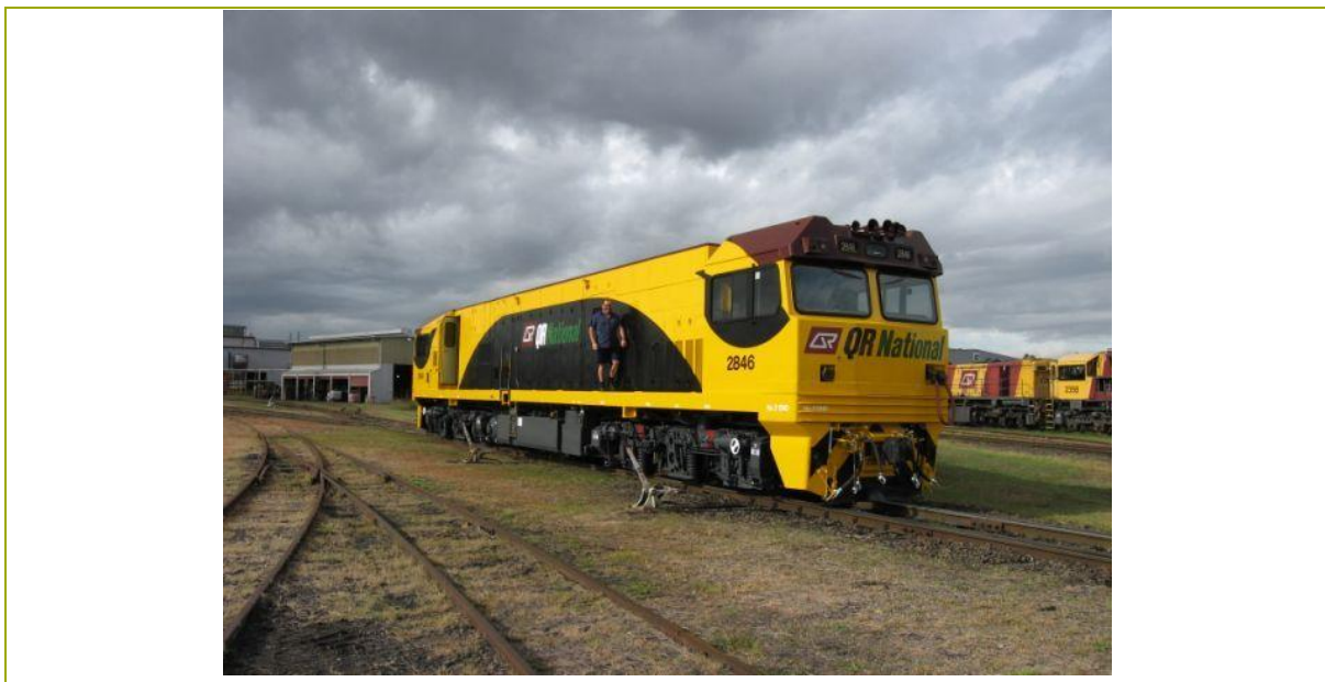
Figure 5.3: A 3,000 Hp 12 Cylinder 4-Stroke Diesel Turbo Locomotive
