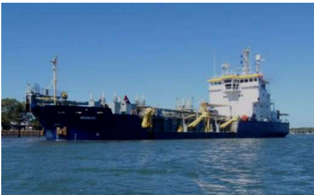
Figure 3: 'Brisbane' trailing-arm suction dredge
