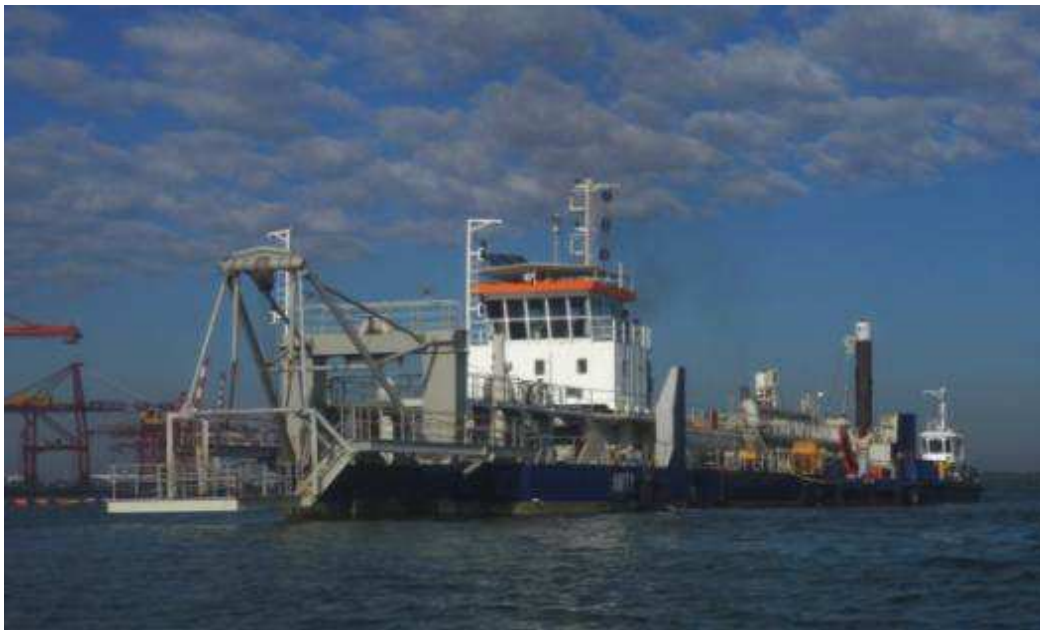
Figure 1: 'Amity' cutter-suction dredge
