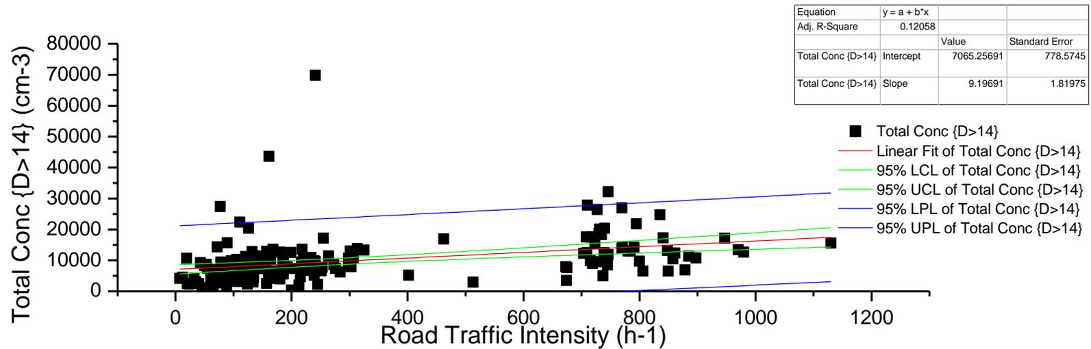
Figure 28: Relationship between Cn and road traffic intensity when winds come from the direction of the road. Also shown are the 95% confidence (LCL and UCL) and prediction (LPL and UPL) limits for the linear model.
