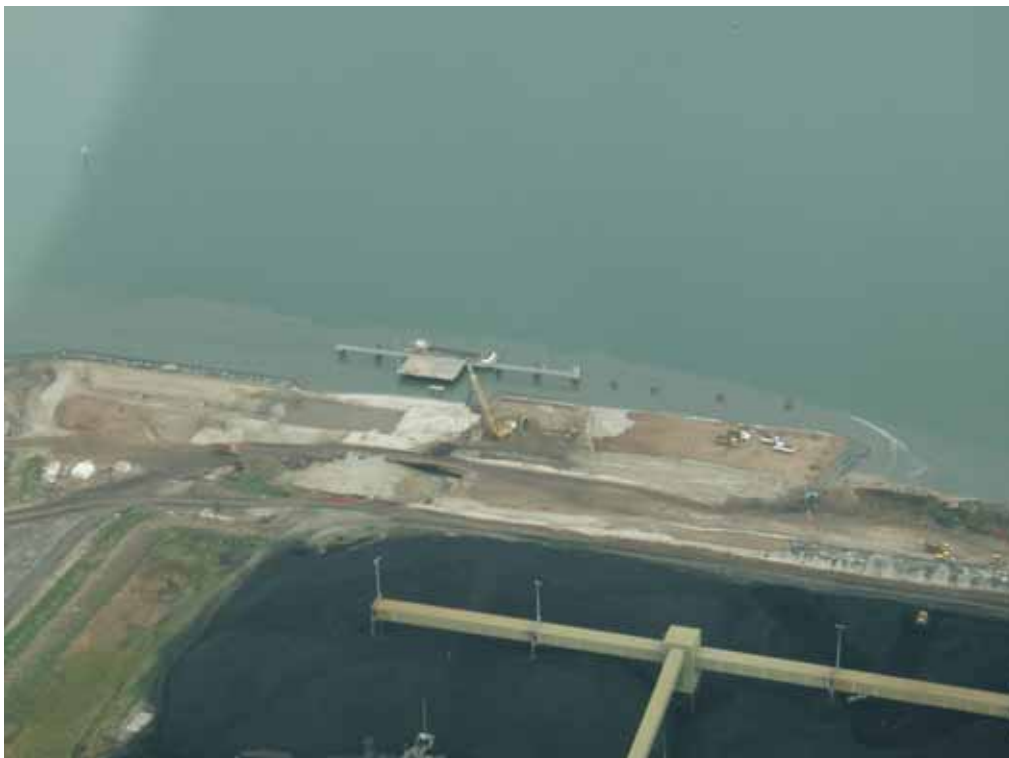
Figure B-5 31 st August 2007 – Turbidity plume associated with the dredge operation of Ken Harvey along the general-purpose wharf construction site
