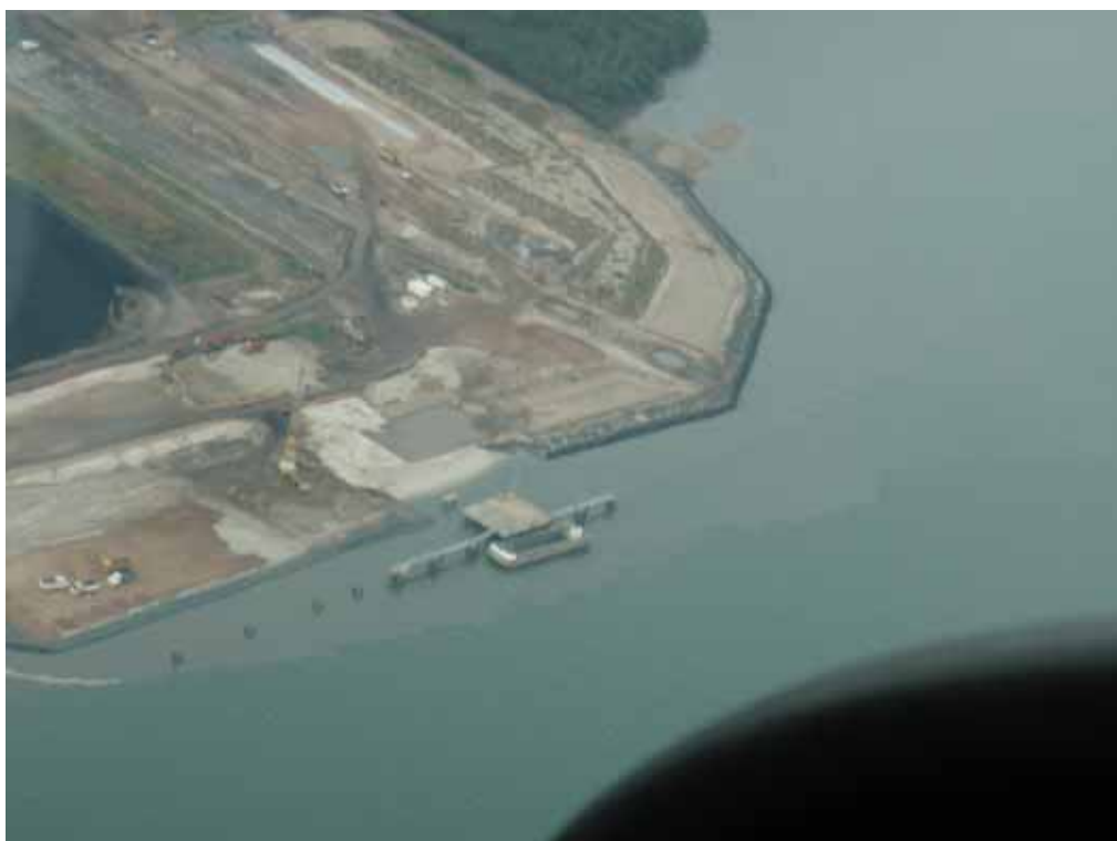
Figure B-6 31 st August 2007 – Turbidity plume associated with the dredge operation of Ken Harvey along the general-purpose wharf construction site
