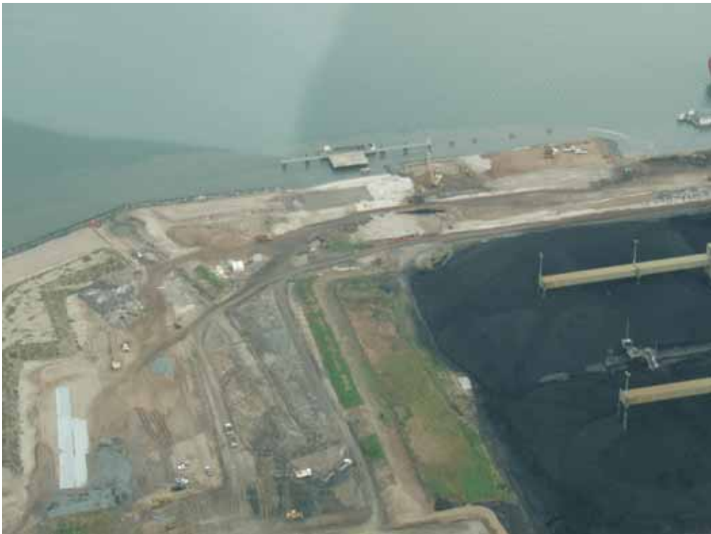
Figure B-4 31 st August 2007 – Turbidity plume associated with the dredge operation of Ken Harvey along the general-purpose wharf construction site
