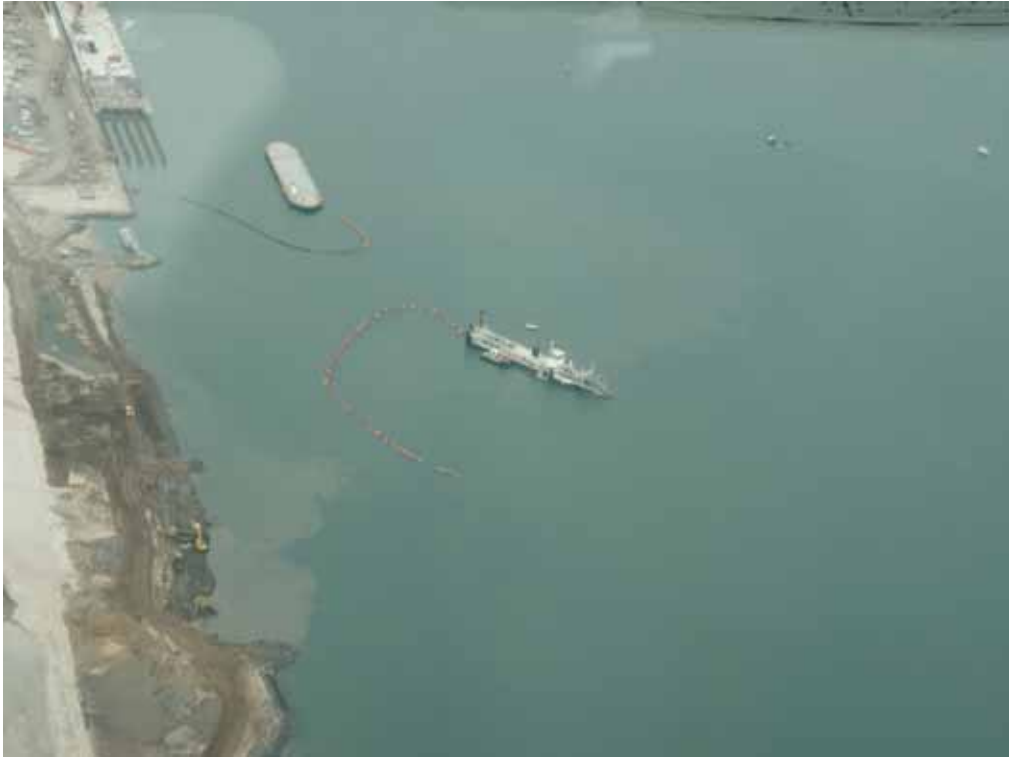
Figure B-3 5 th June 2007 – Turbidity plume caused by earth works within dredging operation
