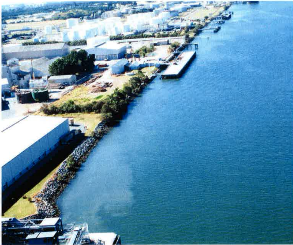
Plate 9: Photo looking downstream from the Pinkenba Bulk Wharf. Turbid plume in shoal water close to shore, downstream of the Pinkenba Bulk Wharf, is associated with a drain discharge and not the bed levelling operations. Drain is located at the mangrove line shown in centre of photo.
