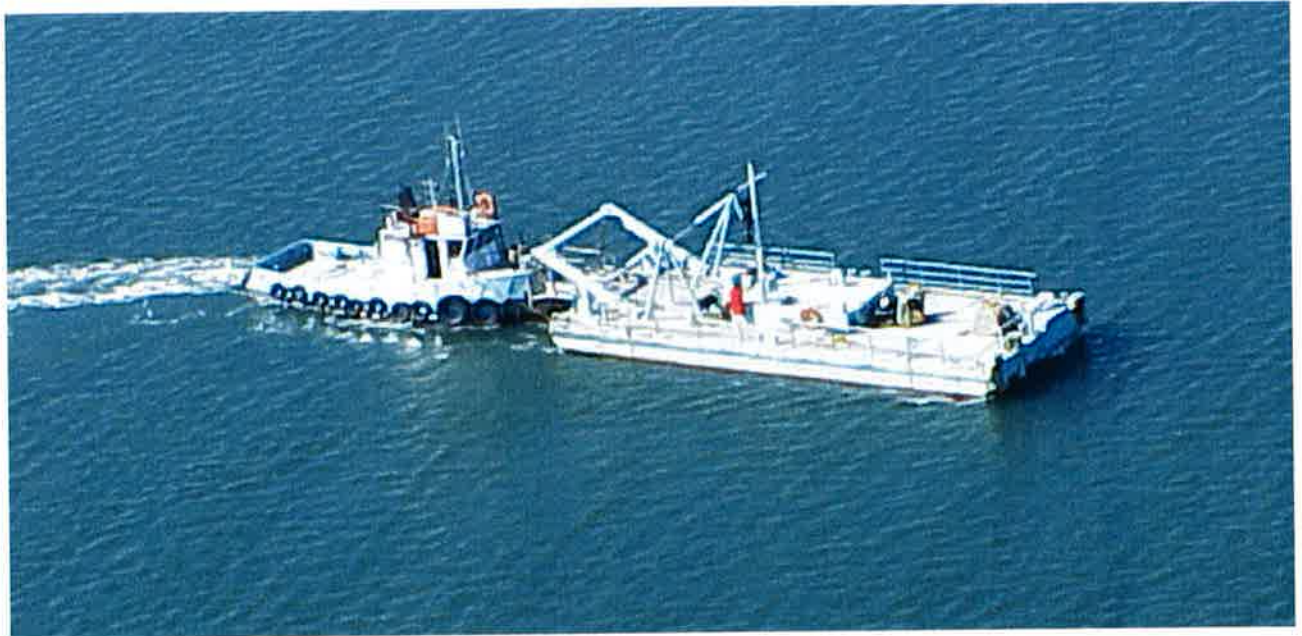
Plate 1: Tug Seahorse and bed levelling barge. The bed-levelling blade is deployed from the gantry at the stern of the barge.
