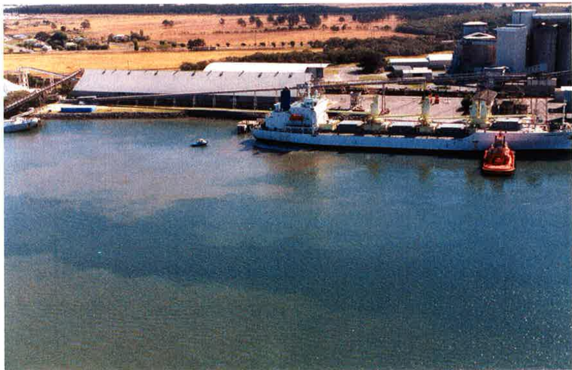
Plate 6: Shown for comparative purposes, the turbid plume created by ship berthing operations at the Pinkenba Bulk Wharf, just upstream of the Incitec North Wharf. Note the turbidity and the extent of the plume were much greater than that associated with bed levelling operations. Plume in foreground of photo was associated with the turning of the ship head to sea, prior to berthing.
